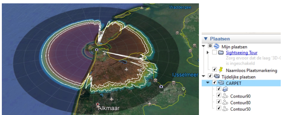
Figure 16: Left: PPI-view diagram of the single scan detection probability, projected on Google Earth. Right: Menu that enables switching on/off contours.
