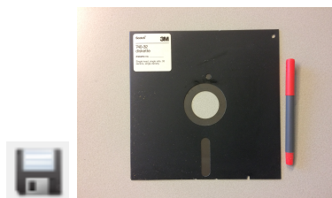
Figure 2.7: Left: File - Save icon, i.e. , a drawing of a 3.5 inch diskette. Right: An 8 inch floppy disk.
