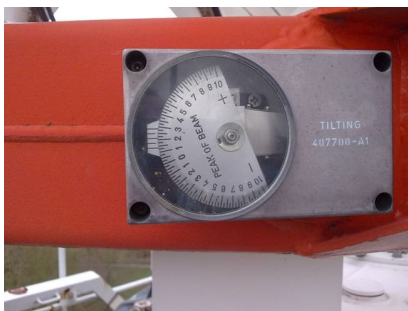
Figure 2.10: A tilting indicator on the antenna of an ATC radar.
