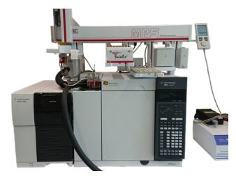
In a GC-MS, components are analyzed using a mass spectrometer (MS) after separation using a GC, facilitating easier identification of the components.
