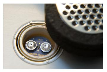
Determination of the heat flow which occurs when a sample is heated, cooled down or isothermally held at a constant temperature under different atmospheres like nitrogen, air, helium or argon. Physical transitions like melting point, phase transition, glass transition and chemical reactions could be determined quantitively. It is also possible to perform a DSC analysis under increased pressure (up to 90 bar) and to follow the DSC measurement visually with a microscope.
