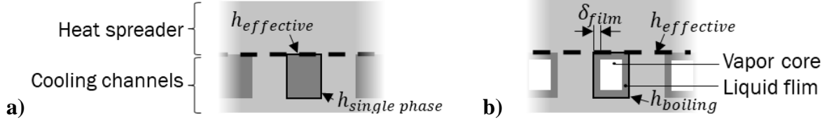
Figure 3. A cross section of the cooling device depicting the plane at which the effective heat transfer coefficient, h_{effective} , is assumed. Two different flow regimes: a) Single phase flow. b) Annular flow boiling.
